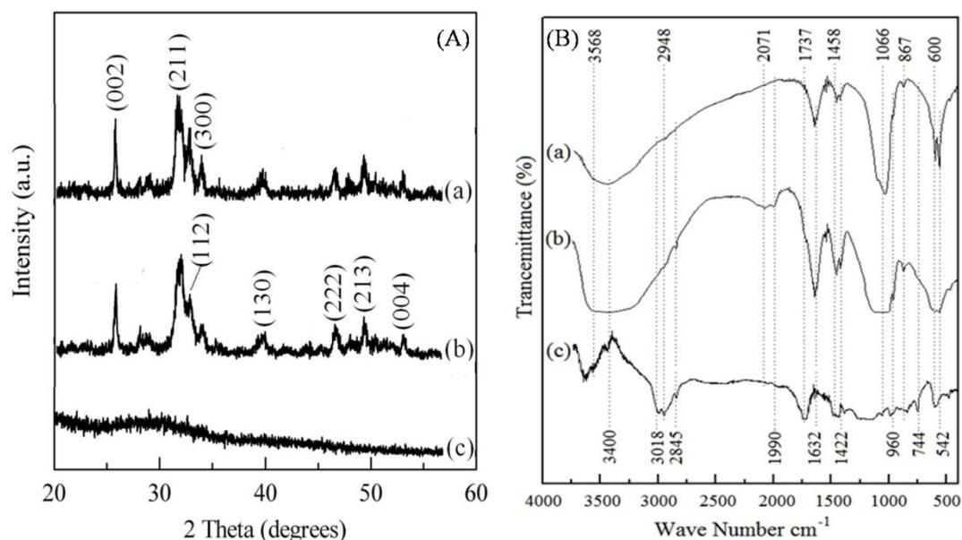
Fig. 1: (A) PXRD pattern of (a) HA (b) HA-PMMA composite (c) PMMA, (B) FTIR spectra of (a) HA (b) HA-PMMA composites (c) PMMA
