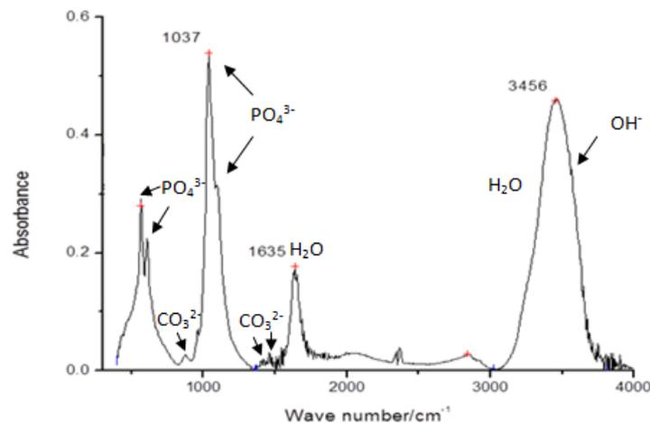
Fig. 3: FT-IR spectrum of synthesized Hydroxyapatite (HA-uSBF)
